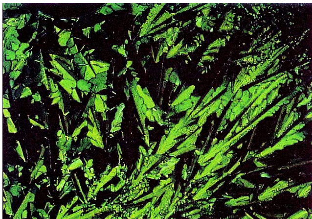
Figure 3. Mesophase texture of the complex (C_{12}H_{25}O)_8PcVO as seen between crossed polarizers at 240^\circ C .
